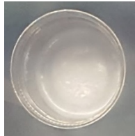
Resolidified Mg(BH 4 ) 2 after 1000 bar, 367 °C
