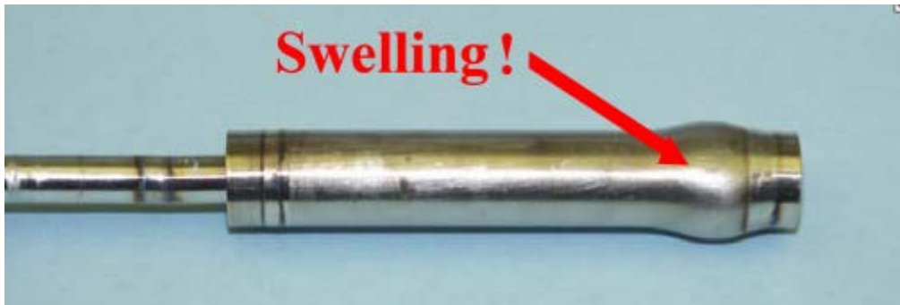
Figure 9. Hydride hydrogen storage vessel deformation caused by material expansion on hydride formation. 51
