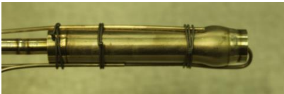
Figure 94. Hydride hydrogen storage vessel deformation caused by material expansion on hydride formation. 51
