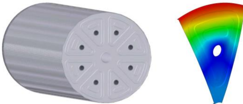
Figure 130. (a) Fin stack showing reinforcing features; (b) example displacement contour plot from FEA to select best reinforcement design. 250
