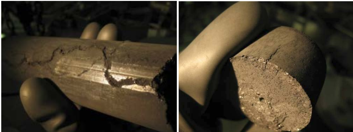
Figure 48. The presence of continuous “wormholes” was observed (left) in addition to discontinuous fissures (right). 100
