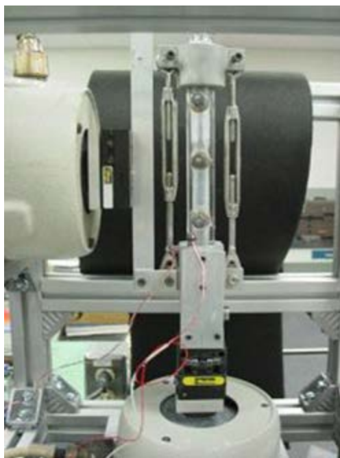
Figure 123. Apparatus with independently controlled, dual axis shakers set up with powder vessel to examine fundamental powder densification characteristics. 250
