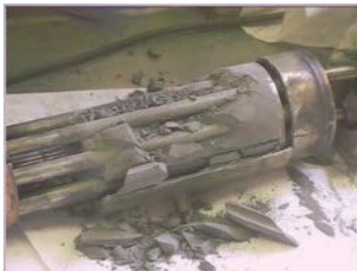
Figure 82. Mg/MgH 2 powder compaction during cycling experienced in the reactor studied in reference 185. 186
