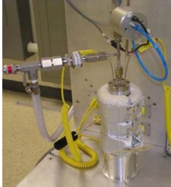
Figure 88. Sample holder attached to the hydriding system. 197
