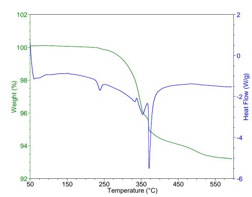
TGA-DSC analyses of hydrogenated MgB<sub>2</sub>-10 mol% graphene
