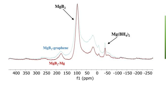
Confirmation of Mg(BH<sub>4</sub>)<sub>2</sub> formation in modified materials hydrogenated at moderate conditions
