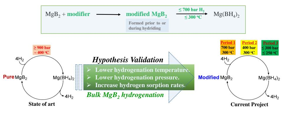
Towards improving hydrogen storage properties of MgB<sub>2</sub>/Mg(BH<sub>4</sub>)<sub>2</sub> system.
