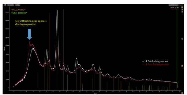
XRD taken in Dera Lab (UH) using single-crystal diffractometer with IuS 3.0 Ag  $K_{\alpha}$  microfocus source.
