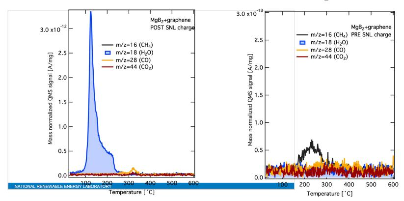
The water impurity is attributed to residual physisorbed  $H_2O$  inside the TPD sample vial.
