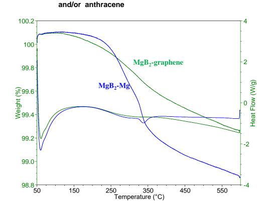
TGA analyses indicates less than 1 wt% hydrogen release
